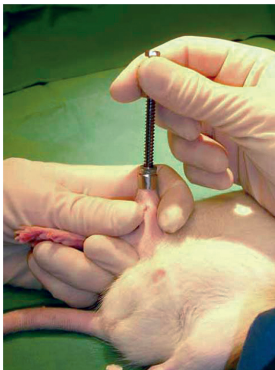
Figure A. The piston was pressurized by a dynamometer with a transcutaneous force of 8 N at 0.17 Hz.
